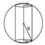
Form the given figure, we have  $h = 2\sqrt{R^2 - r^2}$ The volume (V) of the cylinder is given by,
